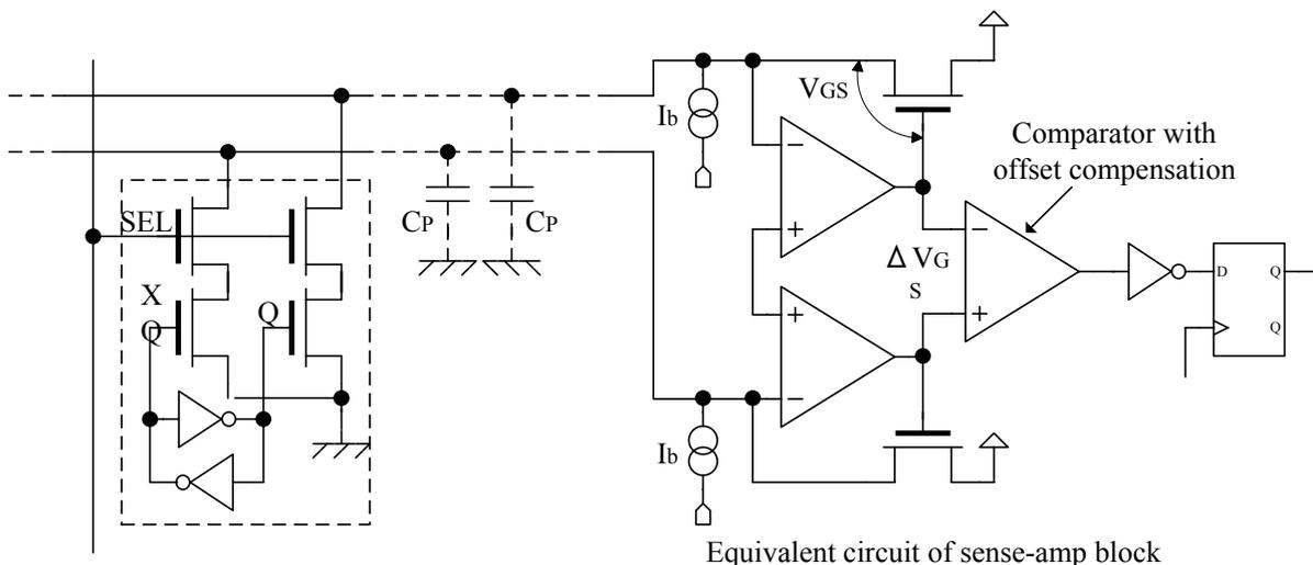
Column A/D Data Readout Sense Amplifier Equivalent Circuit
