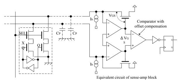
Column A/D Data Readout Sense Amplifier Equivalent Circuit
